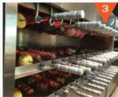
Churrasco skewers shift over to a bigger & heated fire Churrasco machine
